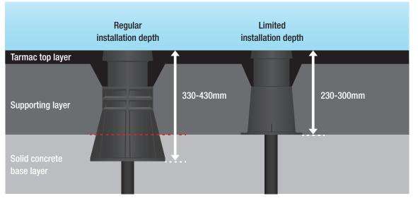
Since many years, AVK is one of the frontrunners in the development, production and sales of height adjustable surface boxes. A suitable solution for installation in tarmac.
