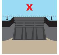
Potential issue 1: tarmac and ground layers sink, surface box doesn't sink enough and rises above road level, leaving a bump in the road.
