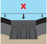
Potential issue 2: surface box sinks faster than road level, leaving a hole in the road
