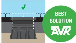
Perfect installation in tarmac road due to flexible top part. The best AVK solution for installation in tarmac.
