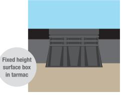
Installation of fixed height surface box in tarmac road. In the situation displayed above it is perfectly aligned with the road surface, but in practice it is often installed too high or too low.
